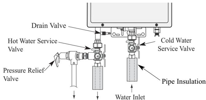
For increased energy efficiency, use pipe insulation. Please install the insulation according to the diagram above, making sure
