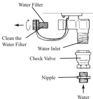
**Notice:** Use only teflon tape on cold and hot water connections and lines.
