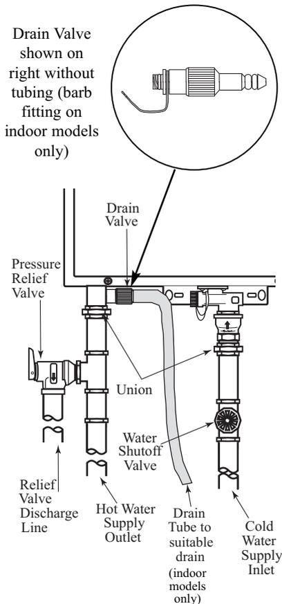
**Notice:** The above illustrates a pressure-only relief valve. If local codes require a combination temperature and pressure relief valve be installed, an extension piece may be needed to ensure that the valve probe is not directly in the flow path of the water.
