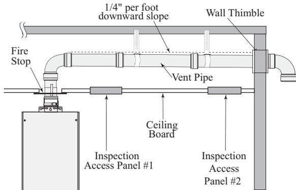
If the vent piping passes through a closed space, a minimum clearance of 8" (20 cm) when installed horizontally or 6" (15 cm) when installed vertically should be maintained between the vent pipe and combustibles and noncombustibles. Be sure to follow local codes and vent manufacturer's installation instructions.
