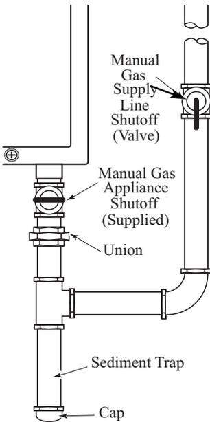
The supplied Manual Gas Appliance Shutoff Valve must be installed at the gas connection of the water heater at the time of installation (see diagram to the left).
