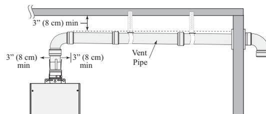
Proper operation of the water heater requires air for combustion and ventilation. Provisions for combustion and ventilation air must comply with referenced codes and standards.
