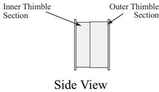
An approved 4 inch (10 cm) Vent Horizontal Wall Thimble must be used.
